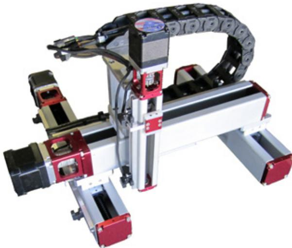
Gantry Systems are a further refinement of a multi-axis solution from **USAutomation** where a complete system is designed as a turnkey solution. Gantry systems generally consist of an underlying X axis, normally with two axis in parallel for moment loading considerations, a spanning Y axis, and a vertical Z axis holding the workpiece or load.
